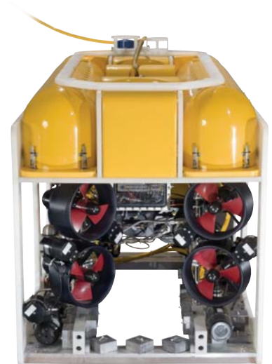
PANTHER-XT PLUS SHOWING TOOL SLEDGE COMPARTMENT
